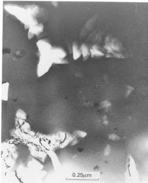
Figure 13 Bright-field transmission electron micrograph of amorphous \text{Fe}_{78}\text{B}_{13}\text{Si}_9 after 30 min at 450^\circ\text{C} .
